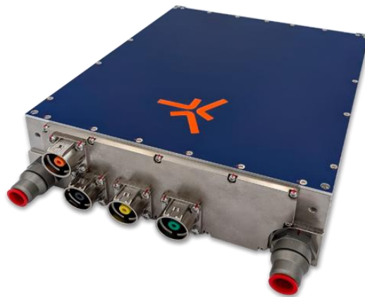
Figure 1 – BrightLoop DC Galvanic Isolator 240 A / 220 kW, up to 1000 V DC , 32 x 28 x 8 cm, <17 kg 30 kW/L and 13 kW/kg power densities.
